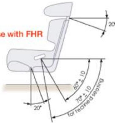
Please also consider when looking at the mounting of harnesses the type of seat being used. FHR also relies on the rigidity of a seat in that a seat with an adjustable seat back or a low backrest may not offer the same level of effectiveness.
